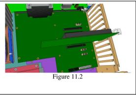
Slide the board down the guide until the edge connect contacts the back plane connector. Press the board firmly into place. Note that the lower end of the metal bracket has to be pushed into a spring clip just below the level of the back plane. This is designed to improve the EMC performance of the system.
