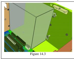
For the ATX model there are a further four retaining screws on the rear of the chassis, while for the Dual Redundant model, there are 8. The ATX model is removed via the top of the chassis however for the Dual Redundant, this is removed via the back as shown in Fig 14.4
