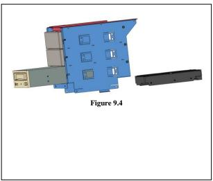
With the drive cage fully removed as indicated in Figure 9.3, there is access to all bays. From Figure 9.4, the HDD is fitted to the bottom 3.5" bay by sliding in from the rear, while for the 5.25" bays, the device is fitted from the front.
