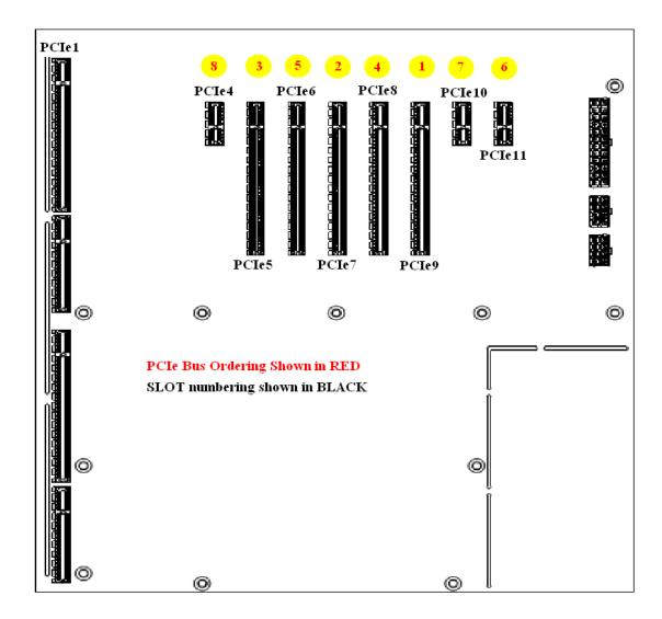
The picture above shows the slot layout on the backplane. Due to the need to match signal lengths between the slots and the PLX 96 lane switch, the slots are not enumerated in order.
