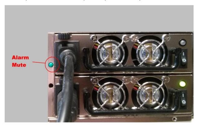
In the event of failure, an audible alarm will sound. This can be cancelled be pressing the Green button shown in the picture above. The faulty module/power inlet will have the LED turned off.
