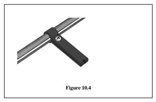
Once the retention arm is secured in place, fit a clamp onto the arm as shown in Fig 10.4. Position the clamp directly over the expansion card to be secured, aligning the small notch on the edge of the clamp with the top edge of the expansion board.
