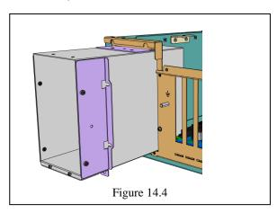
Note that the dual modules are removed first and then the upper bracket is unscrewed first from the inside before unscrewing the remaining 6 screws holding the remaining brackets to the chassis
