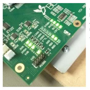
The LED's on the backplane indicate the speed of each PCI Express x 16 slot.
