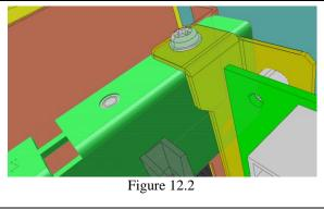
In addition to the retaining screw on the rear panel, the Single Board Computer is held in place with another screw as shown in Figure 12.2.
