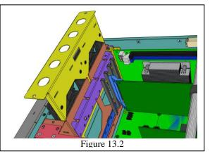
Remove the two retaining screws and pull the fan assembly upwards to remove. Each fan is held in place by 4 screws as show in Fig 13.3 below
