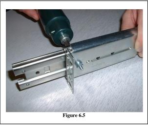
Referring to Figure 6.6 and 6.7, loosely attach the rear bracket to the slide rail outer section. The bracket position indicated is typically suitable for a 600mm deep cabinet. It is recommended that at least two screws, per bracket be used. The screws will be tightened once the slides are installed in the 19in cabinet.
