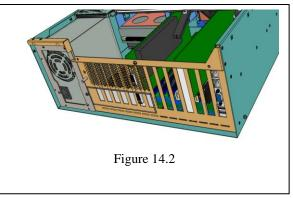
To remove the power supply unit, first ensure that the power supply is switched off and then disconnect the AC supply to the unit.
