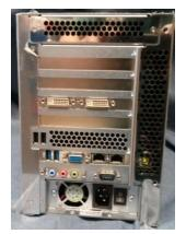
If a Matrox P690 card is fitted, then it will occupy slot number 3 counted from the bottom as shown on the left and on page 2. There are two versions of this card: one with a high density connector requiring an interface cable or one with dual DVI connections (as shown on the left).
