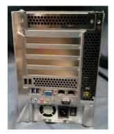
If no additional graphics cards are installed, then the primary display output will be the VGA port on the single board computer, as shown on the left.
