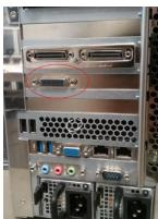
If a Matrox P690 card is fitted, then it will occupy the 3<sup>rd</sup> slot down from the top as shown on the left. There are two versions of this card: one with a high density connector requiring an interface cable (as shown on the left) or one with dual DVI connections.
