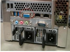
If no additional graphics cards are installed, then the primary display output will be the VGA port on the single board computer, as shown on the left.
