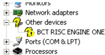
When asked, point the search field to the appropriate USB driver folder: x86 for a 32bit OS and x64 for a 64 bit OS.
