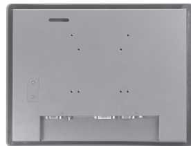
▲ Various mounting ways Panel/Wall/VESA
